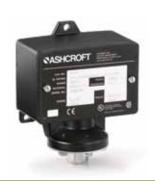
The Ashcroft steam-limit control switch is designed for use on boilers equipped with electrically operated burners. The limit control is an adjustable pressure-operated switch set to stop burner operation when the recommended safe boiler working pressure is exceeded.
