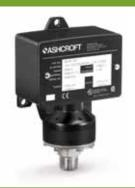
The Ashcroft medium-pressure gas and oil limit control switch is designed for use with air, LP gas, natural gas, #1 and #2 fuel oil and #6 oil preheated to 240°F. This limit control is an adjustable pressureoperated switch with a secondary chamber to prevent fuel from entering the switch enclosure in the unlikely event that the diaphragm develops a leak. The control shuts down a fuel pump in high or low pressure conditions
